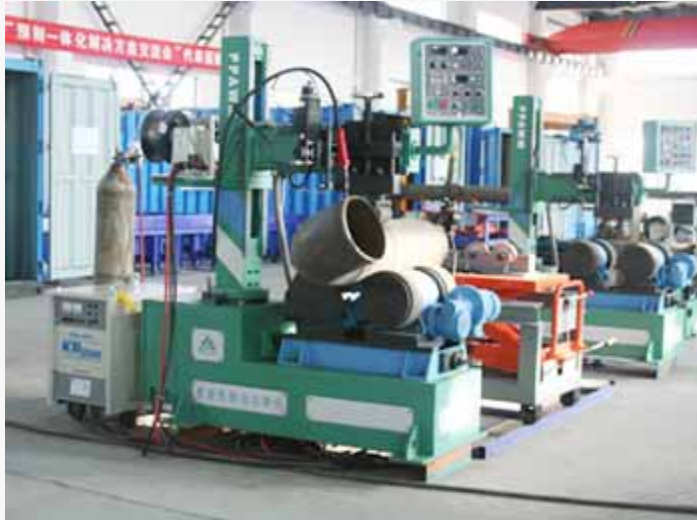
Piping Prefabrication Automatic Welding Machine(FCAW/GMAW)
